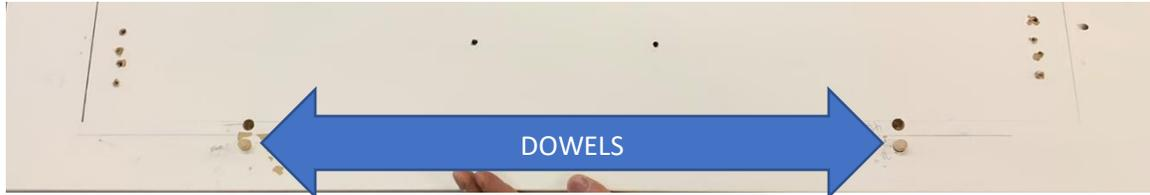
Step 5: Screw the drawer face panel onto the drawer box using the provided screws, do NOT over screw as the MDF inner panel will break.
