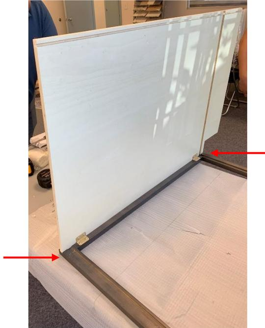
Step 4. Similarly Take the right-side panel to align it on the groove present on back face of the Cabinet Frame. Ensure the top and bottom of the panel is aligned equally to the edge of the frame. Attach the brackets to secure the panels
